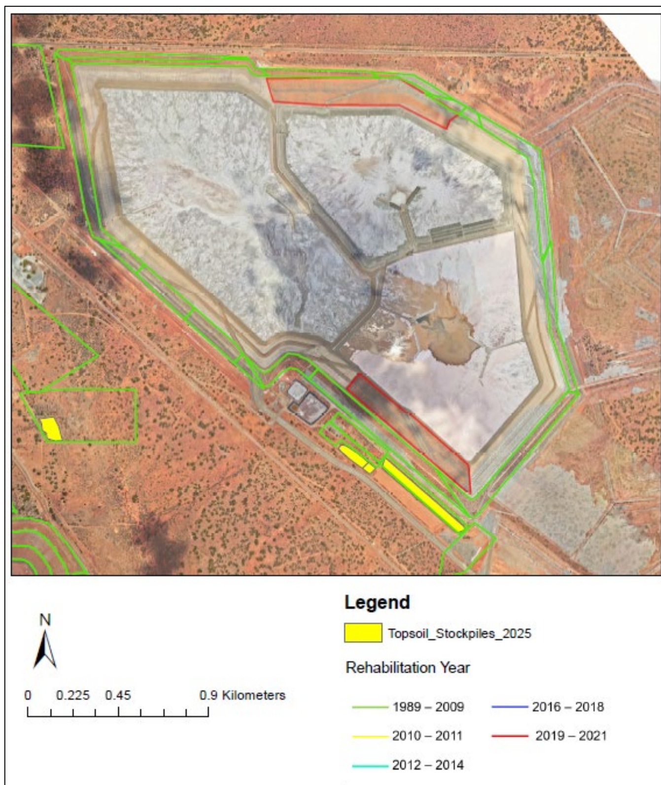
Figure 9-28: Fimiston II TSF current rehabilitation status (2025)
