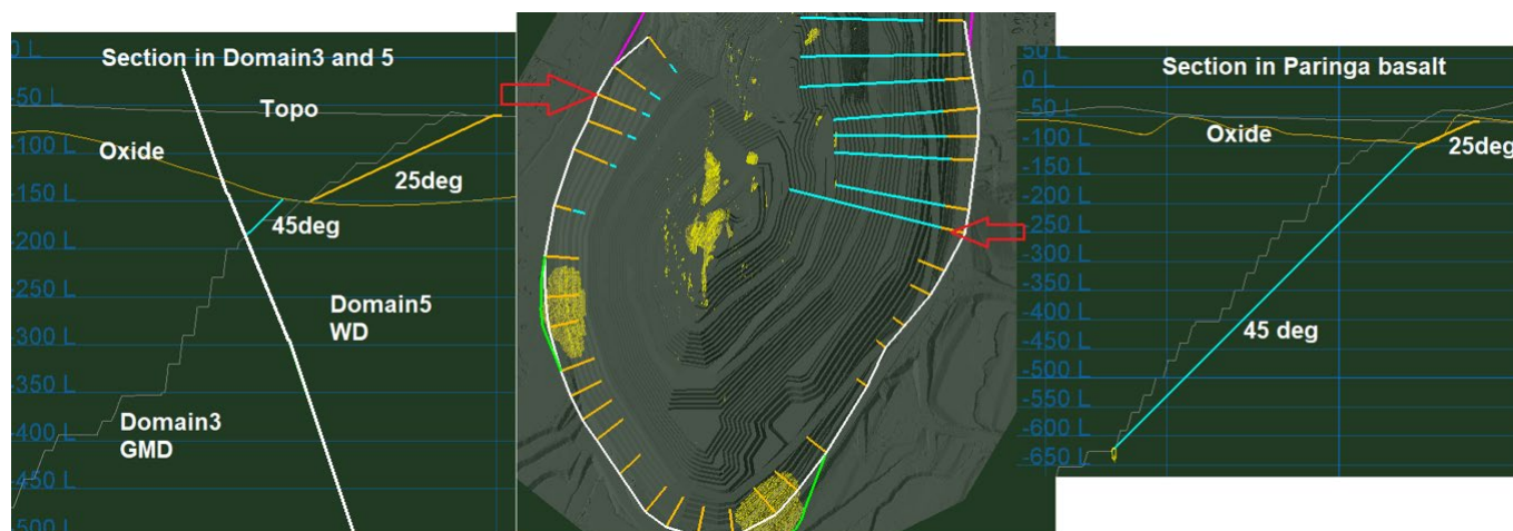
Figure 9-6: Fimiston Open Pit - example of ZOI calculation for the north west wall (GMD)
