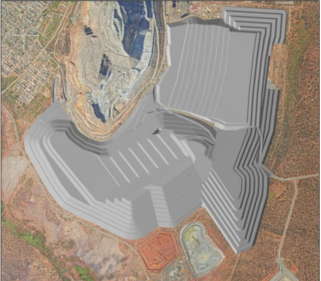
Figure 9-14: Fimiston Waste Rock Dumps Final Design (mine site grid)
