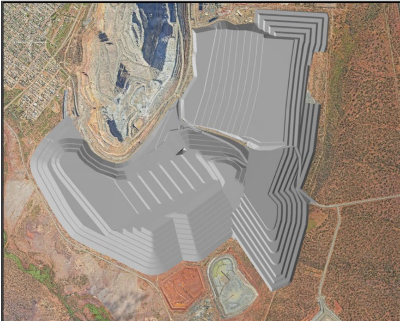
Figure 5-27: Proposed Southern WRD Design (mine site grid)
