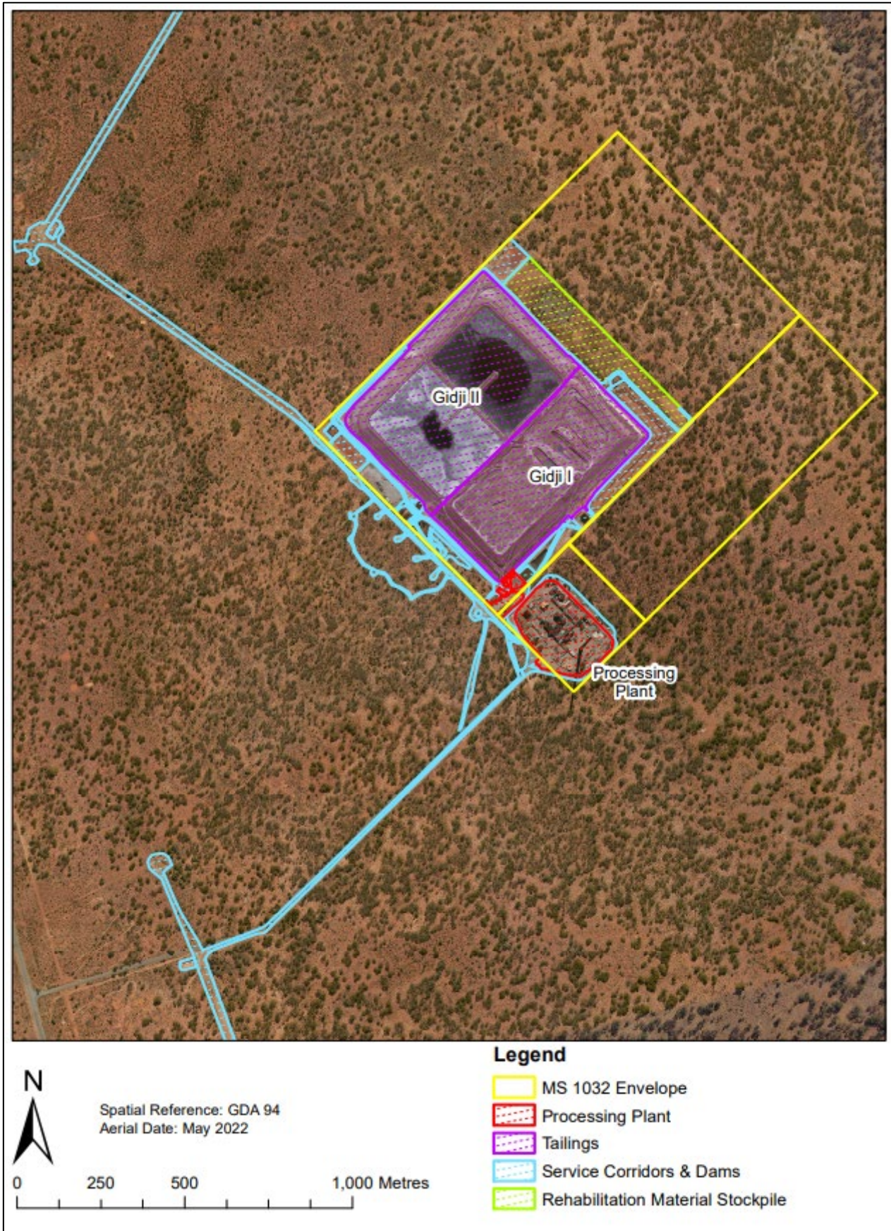
Figure 5-84: Gidji Operational Area, including Processing Plant and Tailings Storage Facility
