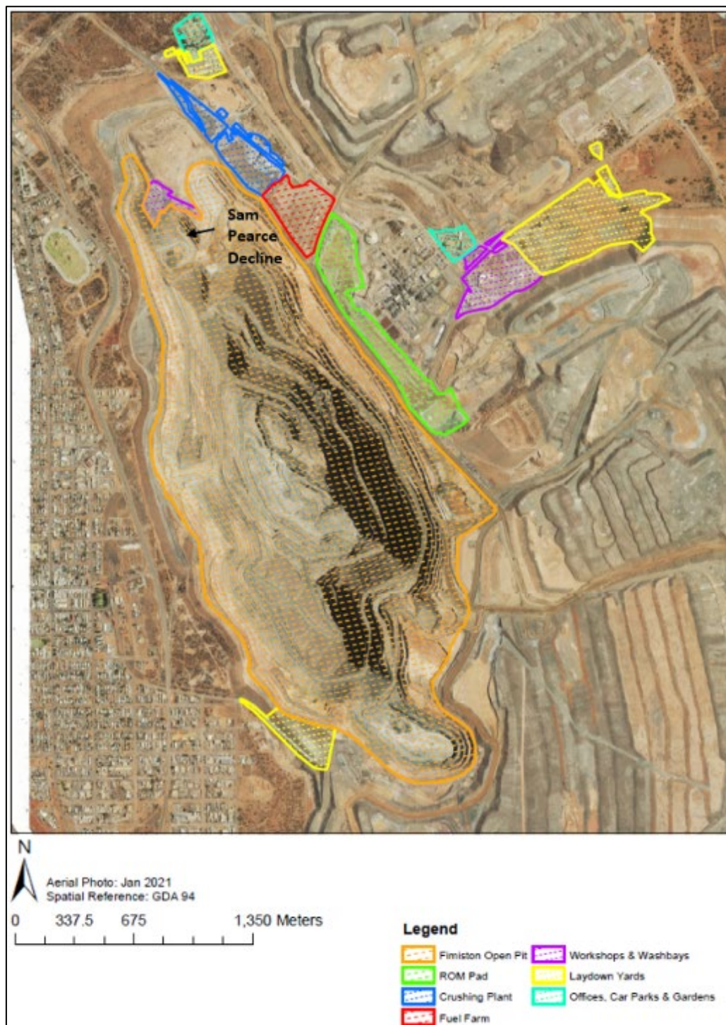
Figure 5-18: Fimiston Mining Infrastructure including Fimiston Open Pit and Sam Pearce Decline (current)
