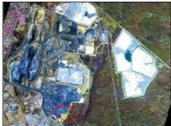
Plate 13: Location of Iron Stained Drainage at Fimiston Waste Rock Dump
