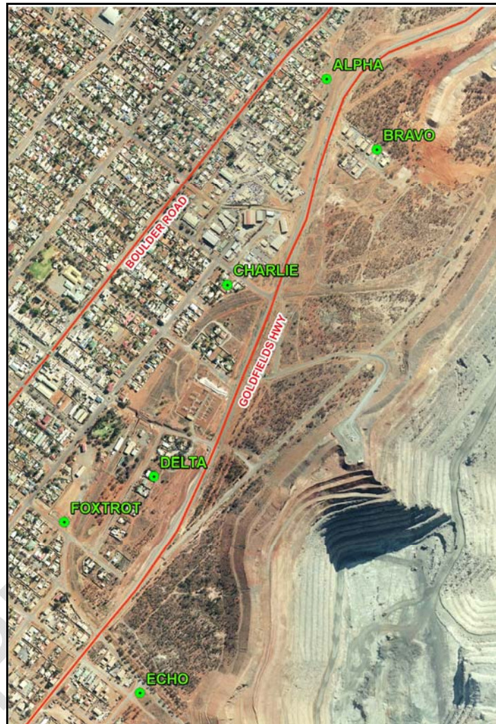
Figure 9 Blast Monitoring Network Location Plan
